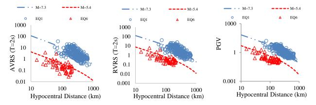
Fig. 2 Results from regression model with recorded AVRS(T), RVRS(T) at T= 2 s and PGV.
