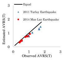
Fig. 5 Regression curve and observed AVRS using maximum (MAX) and geometric mean (GM).
